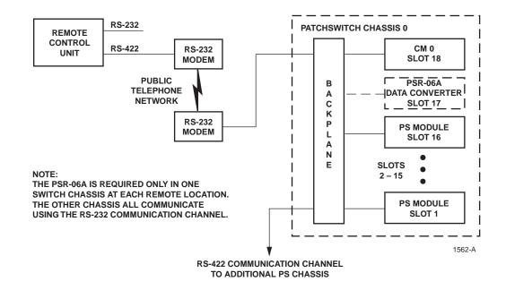
Figure 2-13. RCU to Remote PatchSwitch Chassis
